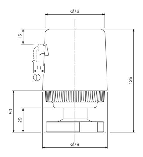
1. Clearance required for electrical cable
