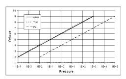
Figure 6 - Voltage to pressure conversion for APG100-XLC
