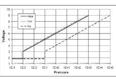
Figure 5 - Voltage to pressure conversion for APG100-XM
