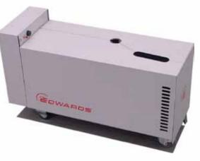
The design of the enclosure allows for it to be easily assembled or disassembled without tooling. A removable front panel also allows for quick access to the oil sight glass. If required a side panel can be removed allowing access to the oil filler cap. The enclosure is powered via a power cable fitting into an IEC 320 socket.
